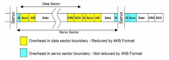
Based on actual Product Format Calculation, the estimated Format Efficiency Gain from 4K-Block Sector is 12-14%, due to the overhead reduction in the data sector boundary, as described in the diagram above (chart courtesy of Hitachi GST).
